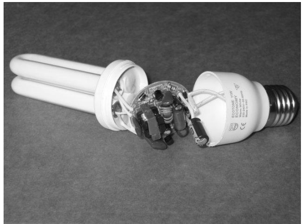
Figure 1: CFL tube, electronics, and base (left to right). Photo from www.pavouk.org/hw/lamp/
